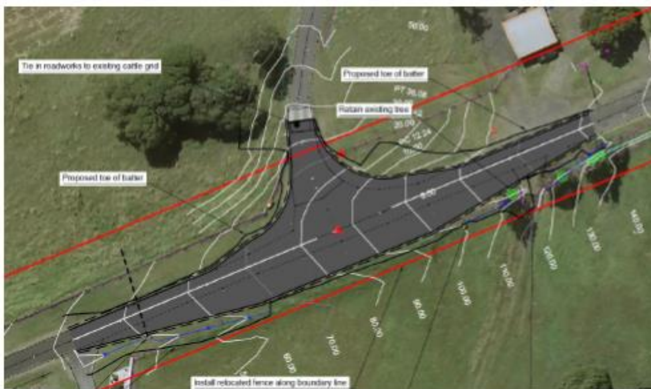
Plate 6: S138 approved intersection works
