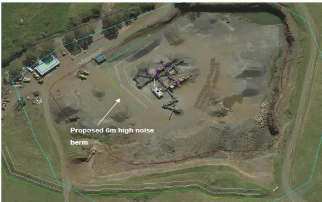
Figure 11 | Proposed noise berm in quarry pit
